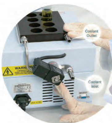
Cooling System Connection Port
