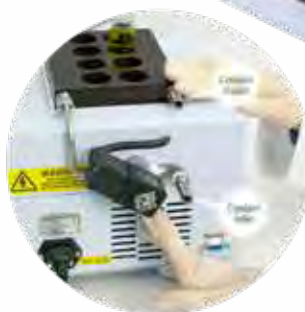
Cooling System Connection Port
